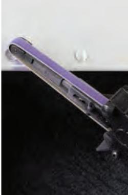
**Rivet/Spot Weld Removal — Belt Grinder**
